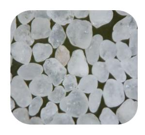
High-purity silica sand from Western Australia with excellent colorability, stable particle size and shape, spherical grain shape, high affinity for resin, contributing to cost reduction in casting production.
